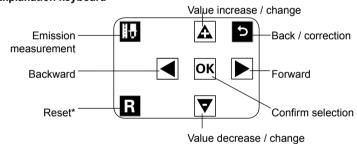
Reset only functions in case of an Error or certain Messages. If reset is rapidly pressed over a short period of time, the device will block completely. Only loss of power (main switch) will restart the device completely. Recommendation: contact your installer and inform them about the fault and give them the number code.
