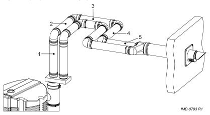
Refer to the table for the correct pipe dimensions of the  ${\rm C}13$  or a  ${\rm C}33$  parallel venting systems.
